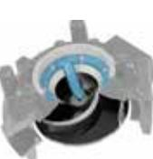
All models with open-channel impeller have an axial adjustment system that maintains the impeller's balance for unchanged pump performance even at first signs of wear.
